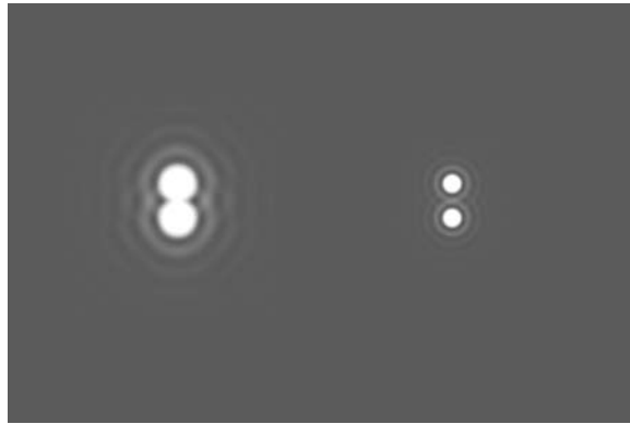
Figure 5.4: A close double star viewed with a 4-inch (10-cm) telescope (left) and an 8-inch (20-cm) telescope (right). Simulated image generated with Aberrator .
