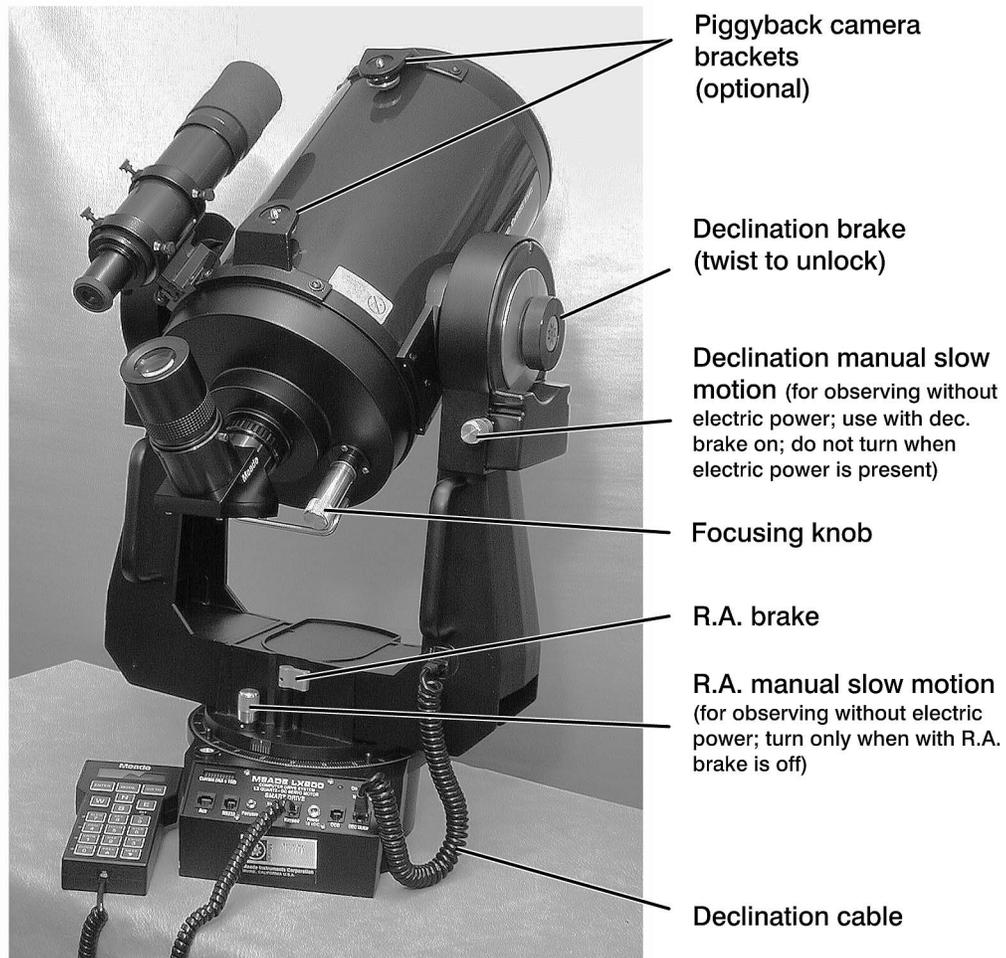
Figure 10.1: Important parts of an LX200 telescope.
